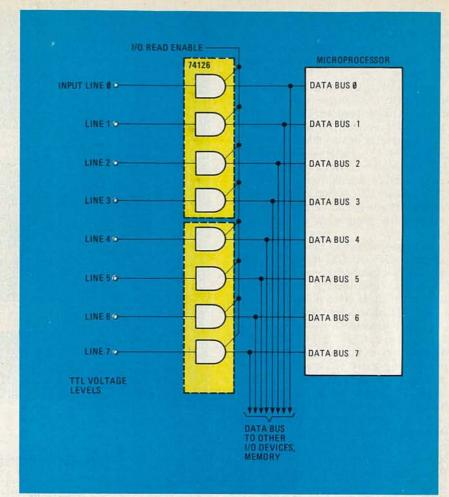
FIG. 6—DISCRETE I/O read logic.
