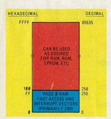
FIG. 3—MEMORY ARCHITECTURE of 8080 and Z80 microprocessors.
