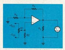
FIG. 8—IF OFFSET-COMPENSATION terminals are not provided, offset nulling can be done using a voltage divider. Here, that divider is connected to the non-inverting input.
