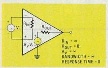
FIG. 3—USING THIS MODEL of an ideal op-amp will make studying the device much easier.
