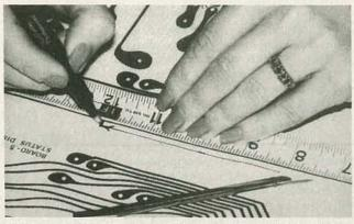
FIG. 7—MARKING OFF a segment of the center line. That segment gives you a useful reference when you make your full-sized mask from your double-sized layout.
