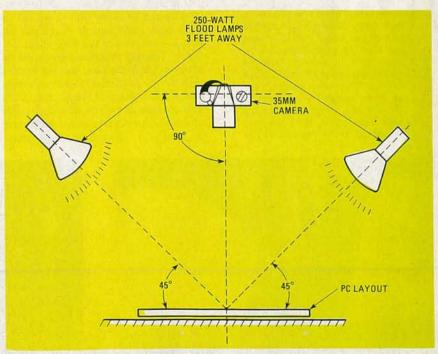
FIG. 11—IF YOU DO NOT HAVE A COPY STAND, you can photograph your layout using the setup shown here.
