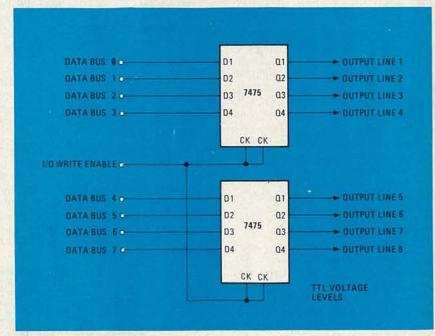
FIG. 7.—DISCRETE I/O write logic.
