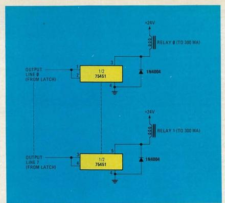
FIG. 8—RELAY DRIVER example.
