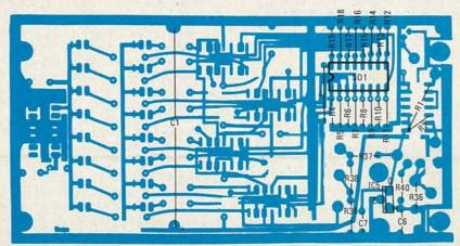
FIG. 6—PARTS PLACEMENT on "foil-side" of display board. Resistor R2 (at right) is soldered to pads on opposite sides of board.
