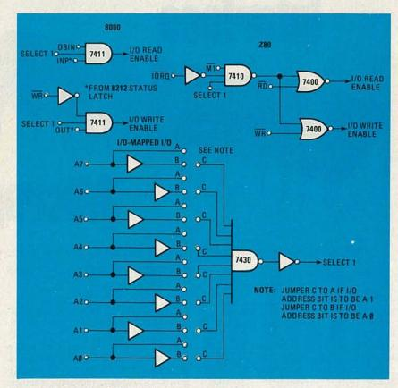
FIG. 4—I/O DECODE for the 8080 and microprocessors.
