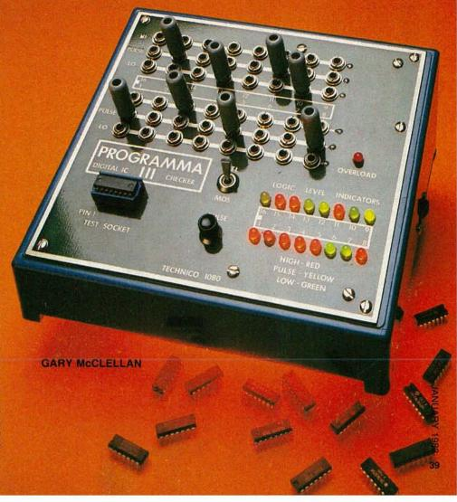
cover that there are only seven IC's in the whole unit! They are all standard, low-cost parts, which makes them easy to find. In addition, this is probably one of the first projects you've seen that uses a VMOS power FET. It does a superior job in the pulse-generator section, and allows pulses to swing the full five-volt range. The display electronics mount on a separate PC board, and simply plug into the panel-board, further simplifying construction.
