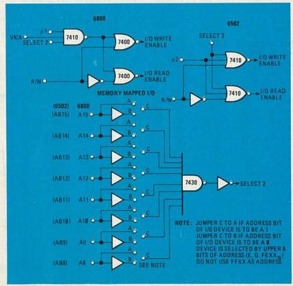
FIG. 5—I/O DECODE for the 6800 and 6502 microprocessors.
