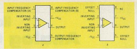
FIG.4—SOME EARLY OP-AMP IC's such as the 709 (shown in a) did not have as much circuitry as later IC's. That's why it had pinouts for such things as input-frequency compensation. Later IC op-amps, such as the 741 (shown in b) have that circuitry built in.
