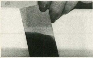
FIG. 12—TO TEST THE DEVELOPER, follow the directions in the text. If it is good, it should turn the film completely opaque.
