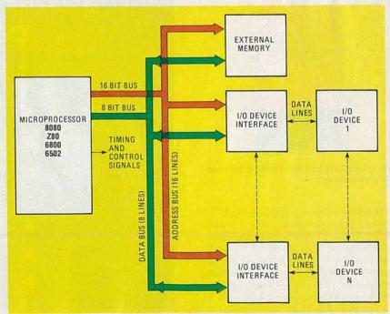
FIG. 1-MICROPROCESSOR system structure.
