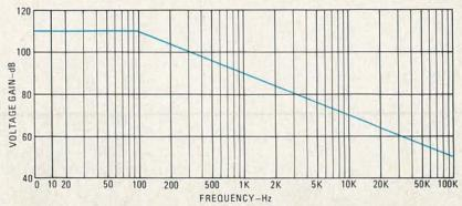
FIG. 10—A FREQUENCY-RESPONSE CURVE, such as the one shown here, can be used to determine the bandwidth of an op-amp. Such curves are often provided on the device's data sheet.
