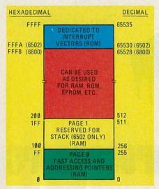
FIG. 2—MEMORY ARCHITECTURE of 6800 and 6502 microprocessors.
