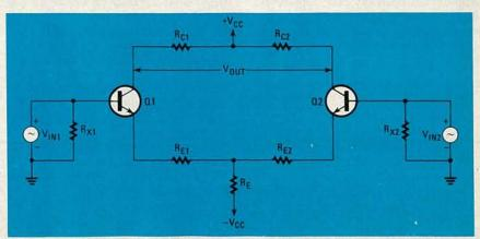
FIG. 1—IN A DIFFERENTIAL AMPLIFIER, the values of R<sub>E1</sub> and R<sub>E2</sub> are often equal to zero.
