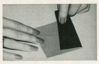
FIG. 9—THE DIFFER-ENCE between the film's emulsion side and base side is easy to see, even when working under a safelight.
