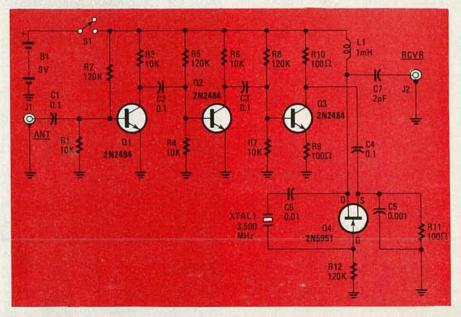
FIG. 2—COMPONENTS USED IN LOW-BAND CONVERTER are readily available. Crystal may be ordered from companies advertising at back of magazine.
